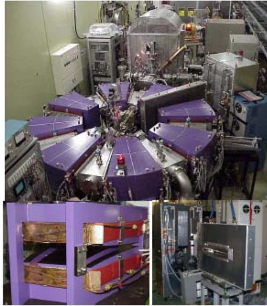
Figure 7: Proof-of-principle FFAG (top). FDF dipole triplet with scaling gap (bottom left) and broad band accelerating cavity (bottom right). [15]
